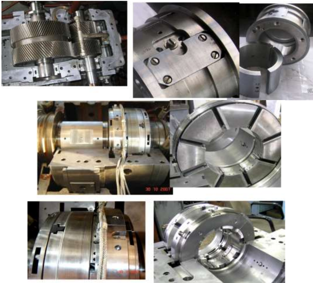
Figure 4 - Damper bearings for multipliers
