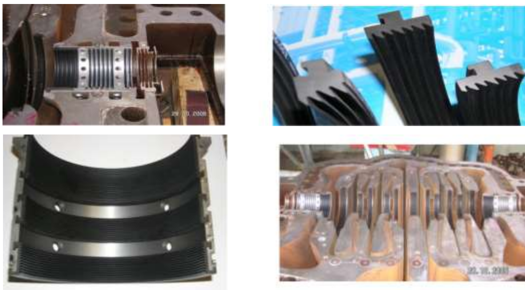
Figure 2 - Labyrinth seals made of polymer material.
