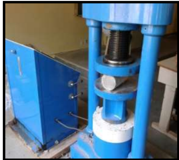
Figure-4 split tensile strength testing of a cylinder
