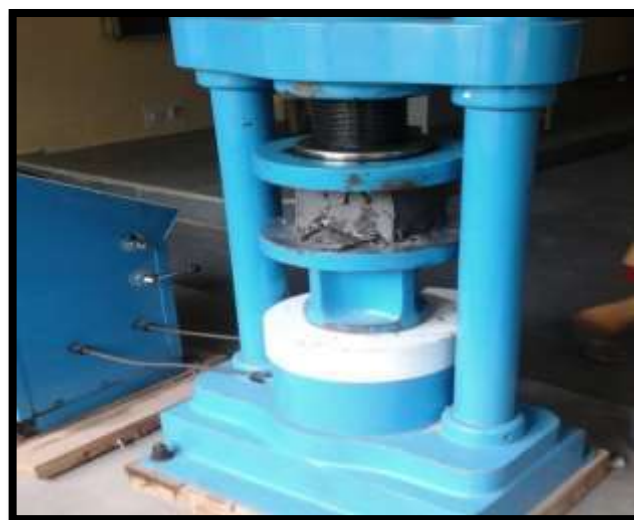
Figure 1: Compressive strength testing of a cube
