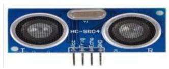
Fig 2.1 Ultrasonic Sensor
