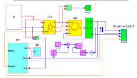
Fig. 1. Mathematical model of the drive in the Simulink environment of the Matlab program.
