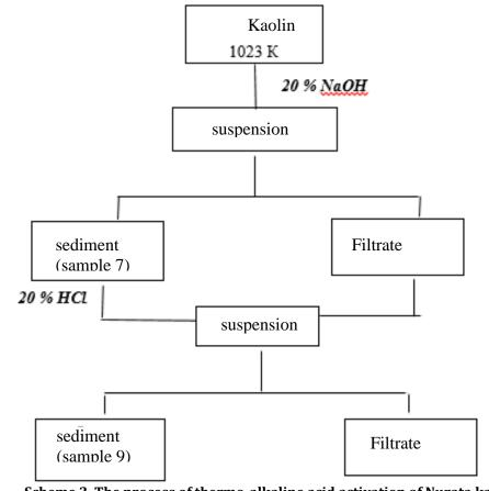
Scheme 2. The process of thermo-alkaline acid activation of Nurata kaolin.
