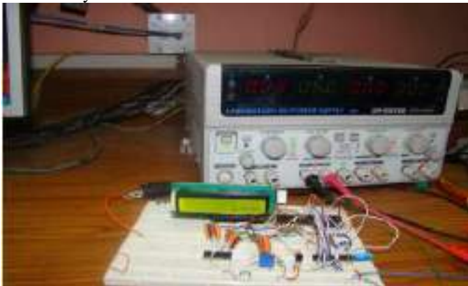
Fig 3. The LCD displaying the room temperature of the lab. The DC power supply is supplying the 5V 0.03A current to the circuit for it to operate.
