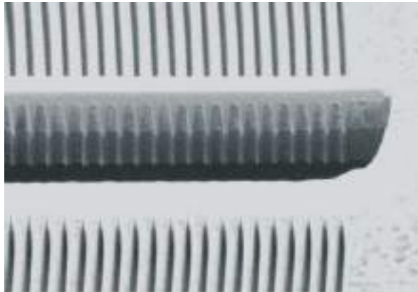
Figure 8: Ion beam cross-section image of outer zones after deposition of a protective and contrast enhancing layer of tungsten [3]
