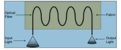
Fig 4: Optical fibers incorporated into a Fabric. Source:Carlos Gonçalves (2018)
