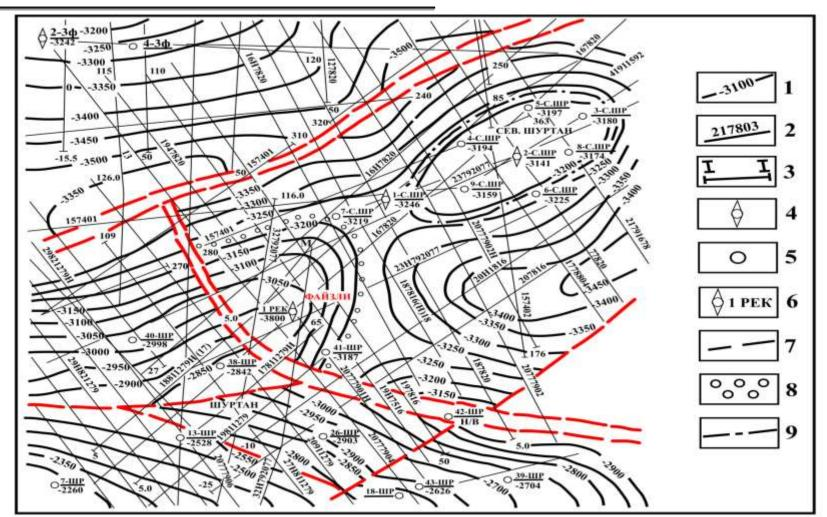
Fig. 2. Structural map on the roof of the lower intercalation chimeric-titenkova layer: 1 – isohypse on Croke lower intercalation; 2 - seismic profiles; 3geological profile; 4 - exploration wells; 5 exploration; 6 – recommended search well; 7 –faults; loop count structure Fazli 9 – VNK. SJIF Impact Factor: 7.001| ISI I.F.Value:1.241| Journal DOI: 10.36713/epra2016 ISSN: 2455-7838(Online)
