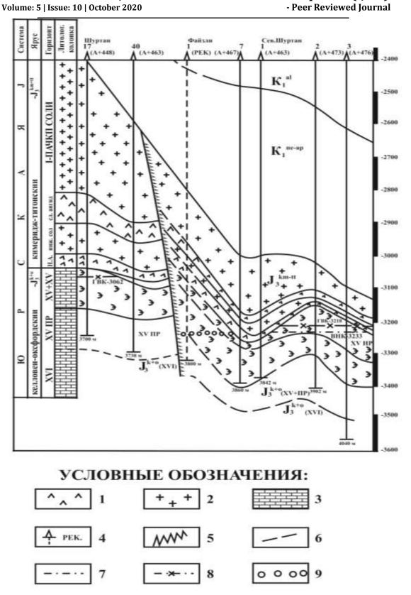
Fig. 1. Geological profile along the line I-I. 1 - anhydrites; 2-salts; 3-riphogenic limestone; 4recommended well; 5 - salt tectonic line; 6-tectonic disturbances; 7 - NVK; 8 - GNK; 9-oil and gas content contour (Faizli structure). ٨
