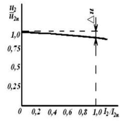
Figure 2. External characteristics of the transformer.
