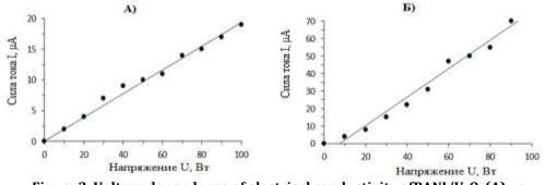
Figure 2. Voltage dependence of electrical conductivity of PANI/V<sub>2</sub>O<sub>5</sub>(A) va PANI/Fe<sub>2</sub>O<sub>3</sub> compositions.
