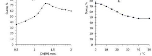
Figure 2. Oxidation to PANI yield: effect of monomer mole ratio (A) and reaction mixture temperature (B).
