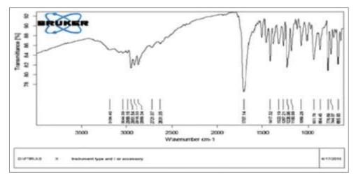
Fig. 1: Fourier transform infrared spectra of ibuprofen
