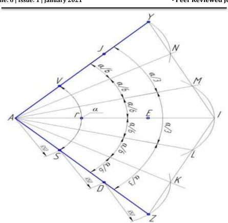
Thus, we can conclude that the division of an obtuse angle into three and six equal parts, is acceptable for accurate graphical construction and making gear sector machine parts.
