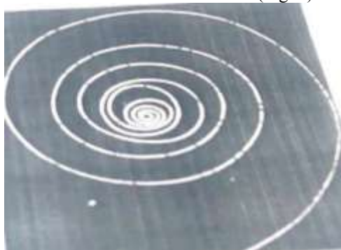
Figure: 3. Trajectory of motion of an electron in a bubble chamber filled with a liquid waterfall.
