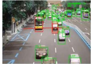
Fig. 4.2: Detection of a traffic violation output frame: bounding box and violation detection (signal jump)
