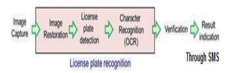
Fig 3.2 : Analysis Model of Traffic Intrusion System
