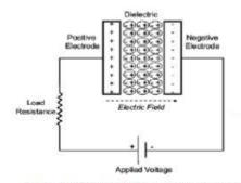
Figure 2.Schematic of a conventional electrochemical double-layer capacitor
