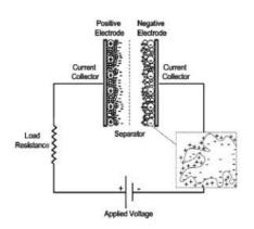
Figure 1. Schematic of a Capacitor
