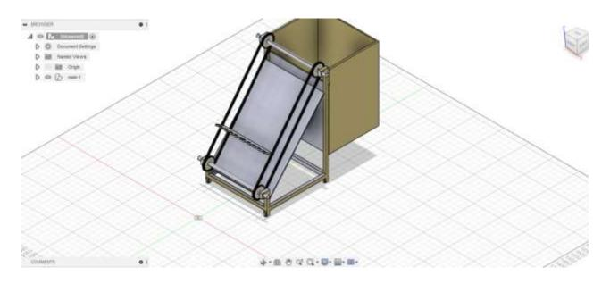
Figure1: CAD Model of Automated Sewage Cleaner (Model created on Autodesk Fusion 360 Software)
