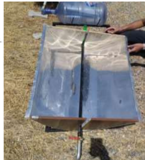
Figure 1. Construction scheme and general appearance of a parabolocylindrical solar water heater.
