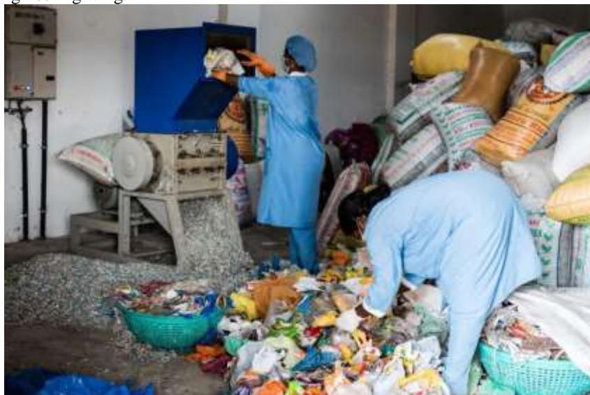
Shredding and sorting plastic waste in shredding units
