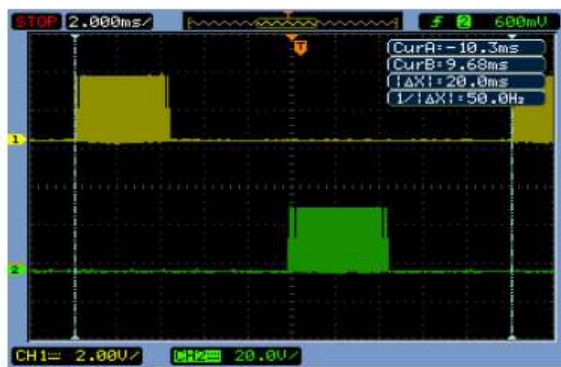
Fig 9.FPGA output of switching signals S5 and S6
