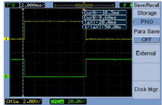
Fig 8. FPGA output of switching signals S3 and S4
