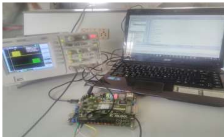
Fig.6.FPGA implement setup using Xilinx SPARTAN6 FPGA kit.
