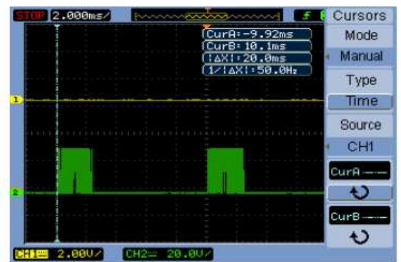
Fig 10.FPGA output of switching signal S7
