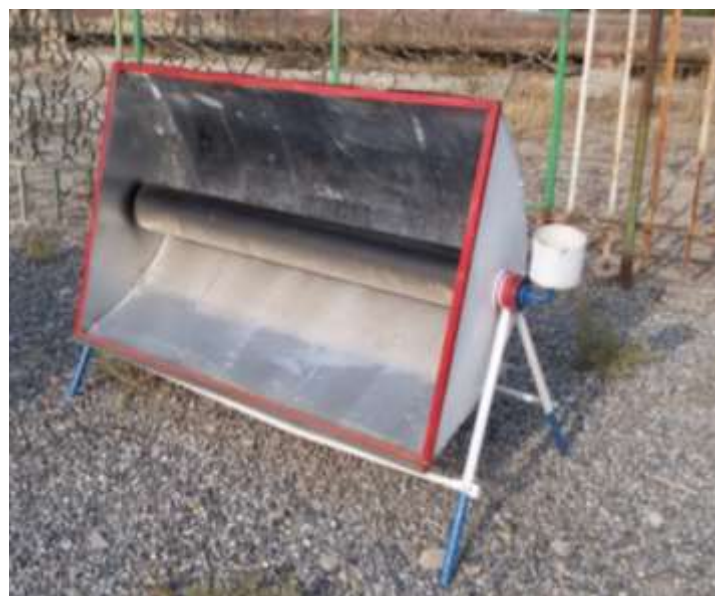
Figure 2. Parabolic cylindrical concentrator with hot water storage accumulator.
