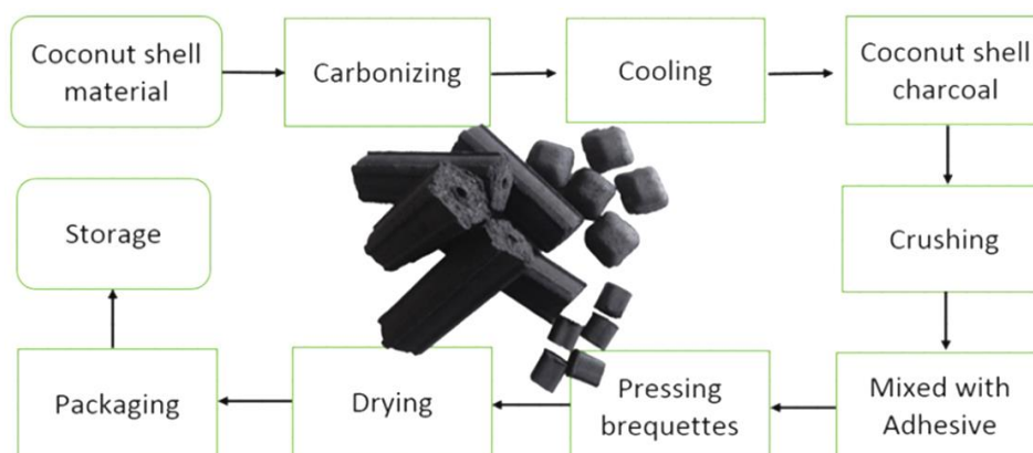
Figure 7. Schematic Diagram of the Process in Developing an Activated Charcoal from Coconut Shell
