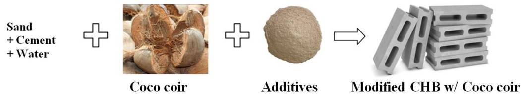
Figure 5. Schematic Diagram of the Process in Developing Modified Concrete Hollow Block with Coco coir
