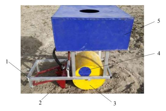
Fig.5. General view of the soil-compacting body: 1-frame; 2-moisturizing body; 3-skating rink; 4-lid; 5-capacity for water. The results of irrigation studies are shown in Table 2.
