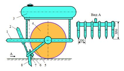
Rice. 2. Hydromechanical sealing device
