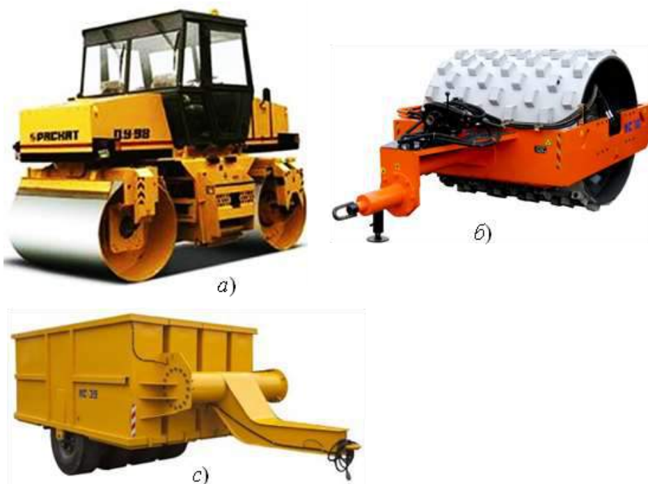
Rice. 1. Machines for soil compaction: a - with a smooth roller; b - cam; with - on pneumatic tires
