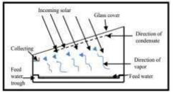
Figure 1.2 Operation of conventional solar stills
