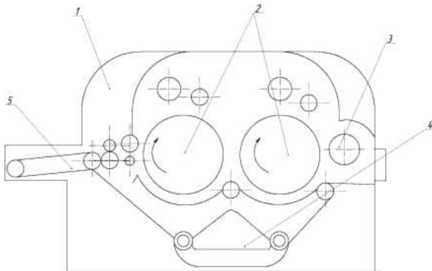
1- chamber, 2- main drums, 3- drums, 4- bunkers, 5- belt conveyors.
