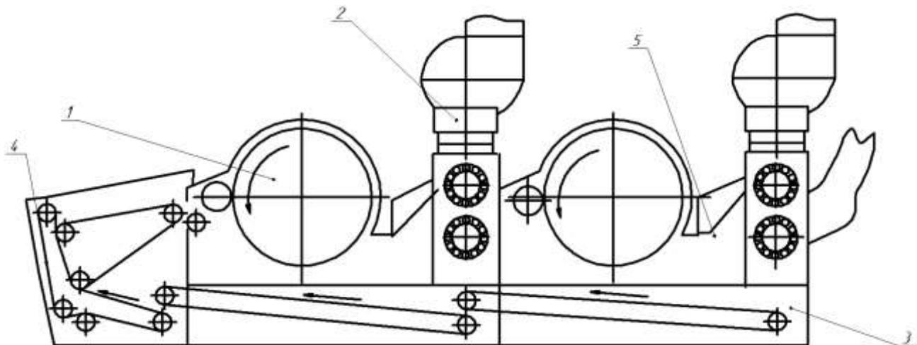
1- main drum, 2- pipe system, 3- belt conveyor, 4 -belt conveyor system, 5- chamber.
