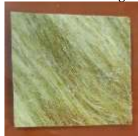
Fig 3.9(b) Final Product Of Cross Ply
