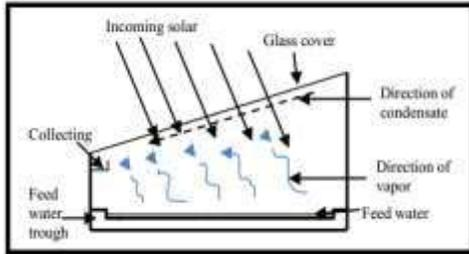
Figure 1.2 Operation of conventional solar stills
