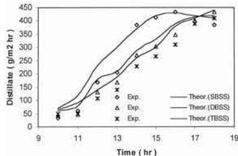
The figure represents the hourly experimental and theoretical distilled output they have found that the
