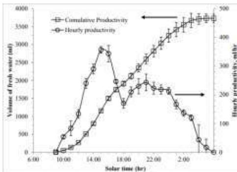
highest daily productivity obtained is 4300 ml and also the effect of water level in basin also studied and its results in operating in lower water level in the basin i.e. 5cm made the temperature of water basin higher than when operating at 8 and 10 cm
