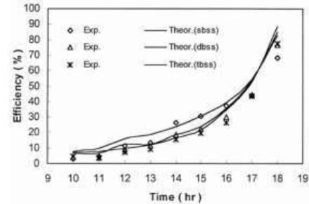
They have obtained that maximum daily efficiency of triple basin, double basin and single basin solar still was 44%, 42% and 32% respectively.
