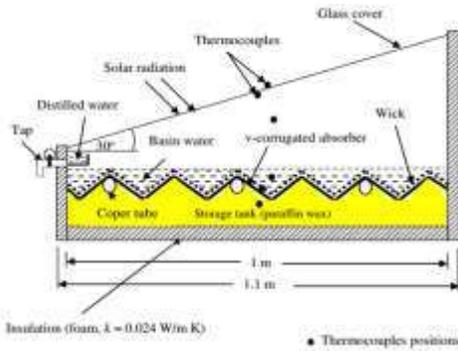
The daily productivity of the still with the PCM when  $m_w = 25 \text{ kg}$  is 12% and 11.7% better than those for the v-corrugated still without the PCM and with the PCM using wick, respectively. Cost analysis is also performed where the cost per liter (CPL) for the still without PCM, with PCM and with PCM using wick are estimated at 0.07182, 0.08369 and 0.09558 \$/l, respectively.
