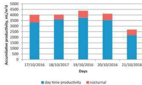
Fig. 17. Variation of the daily and nocturnal productivity of the inclined stepped solar still for the 4th run.
