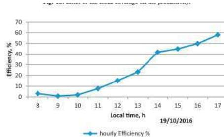
Fig. 16. Hourly efficiency variation of the inclined stepped solar still.
