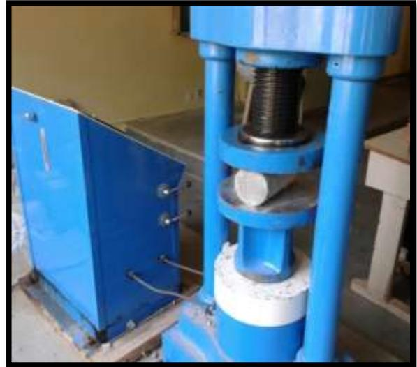
**Figure-4 split tensile strength testing of a cylinder**
