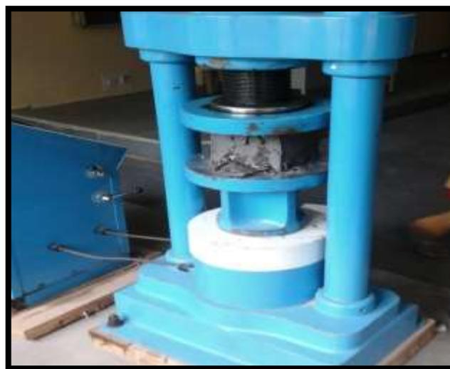
**Figure 1: Compressive strength testing of a cube**
