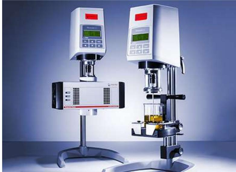
**Fig. 2. Rotational Rheometry.**
