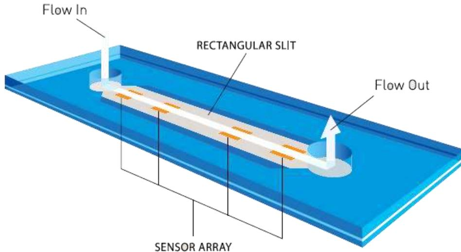
**Fig. 4. Microfluidic device.**
