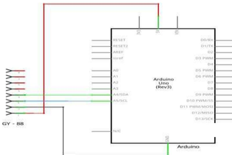
Figure 9. Schematic Diagram of GY-88 Sensor
