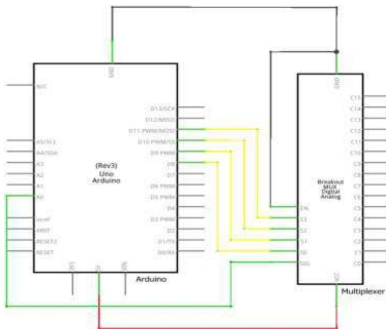
Figure 11.Schematic Diagram of Multiplexer
