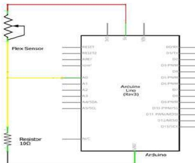
**Figure 7.**Schematic Diagram of Flex Sensor
