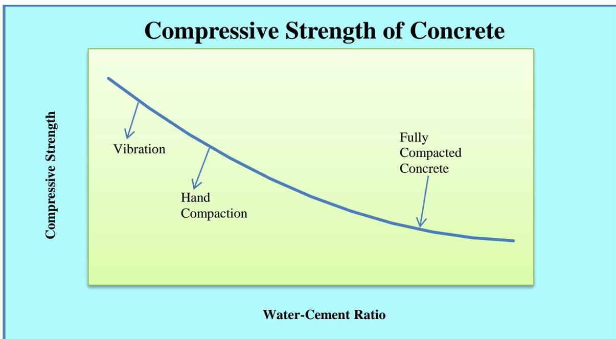
Fig. 1.1. The relation between strength and water-cement ratio of concrete
