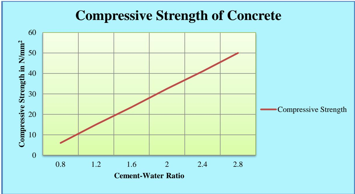
**Fig. 1.2. The relation between strength and cement-water ratio**
