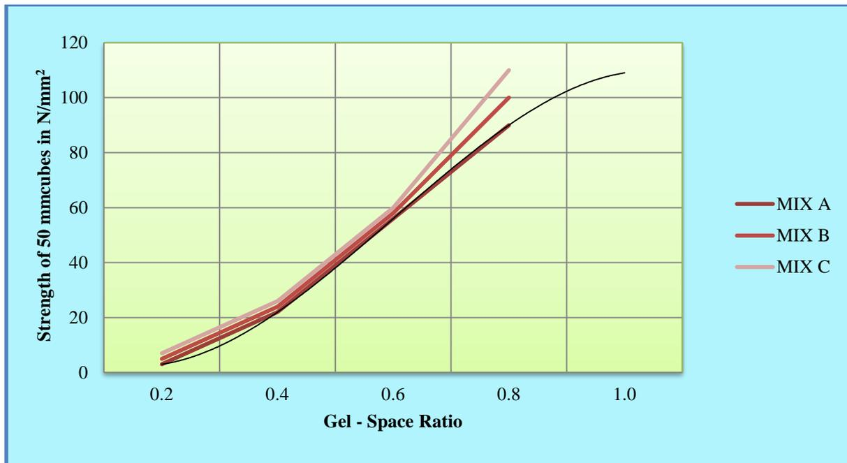
Fig. 1.3. The relationship between compressive strength of mortar and gel-space ratio
