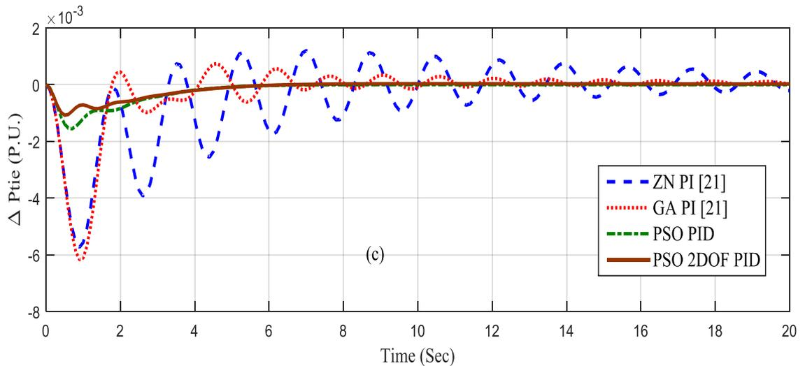
**Fig 1.3 Tie line power deviation for two area thermal and hydal systems**
