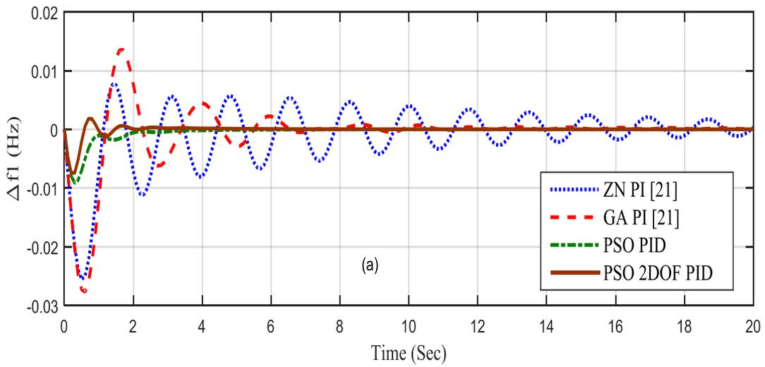
**Fig 1.1 Frequency deviation two area thermal and hydal system at area-1 for load disturbance of 1%**
