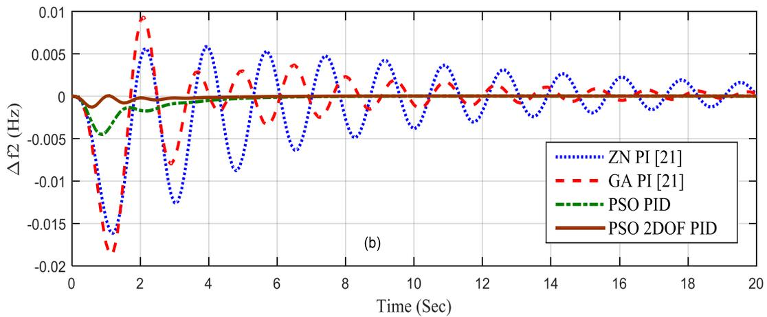
**Fig1.2 Frequency deviation two area thermal and hydal system at area-2 for load disturbance of 1%**
