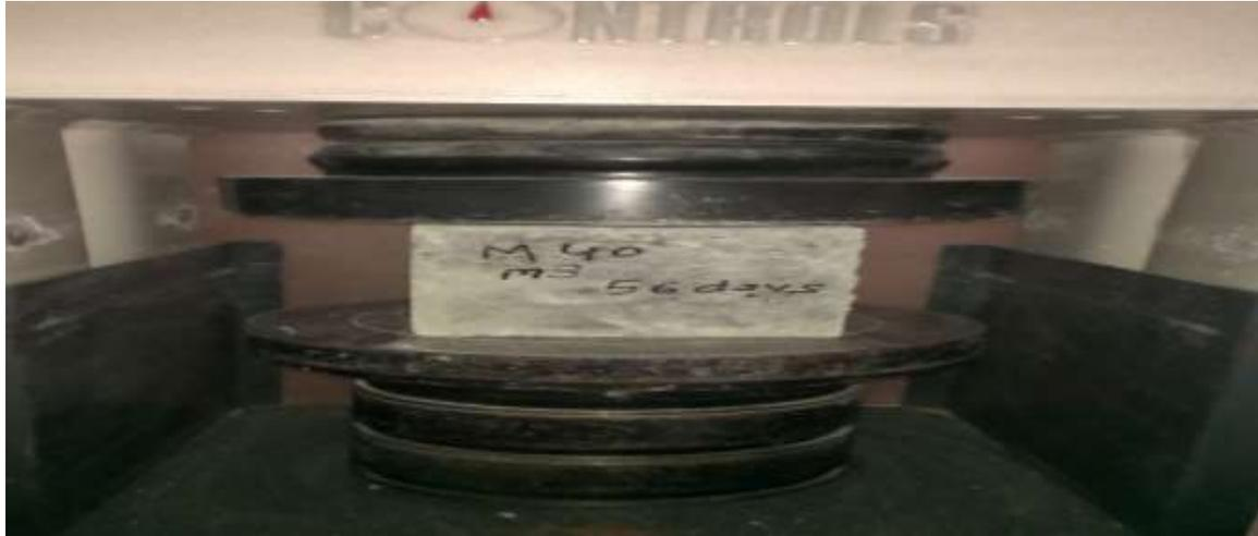
Figure 4.3 Test for Compression Strength In CTM.
