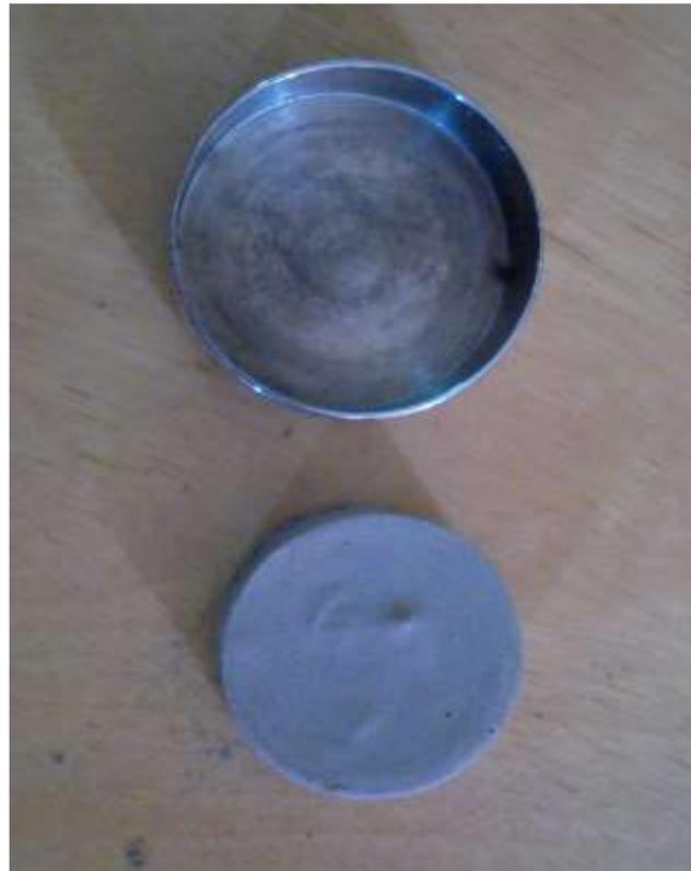
**Figure4 : Shrinkage dish having wet soil pat**
