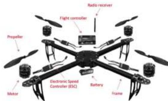
Figure 1. Architecture of a quadcopter
