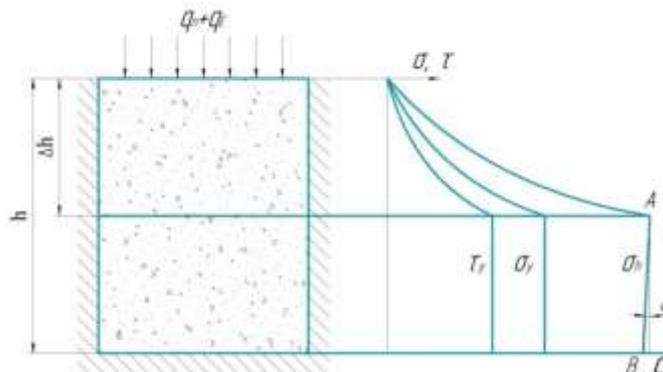
**Figure 2. Scheme of stress distribution during compression of the mixture.**
