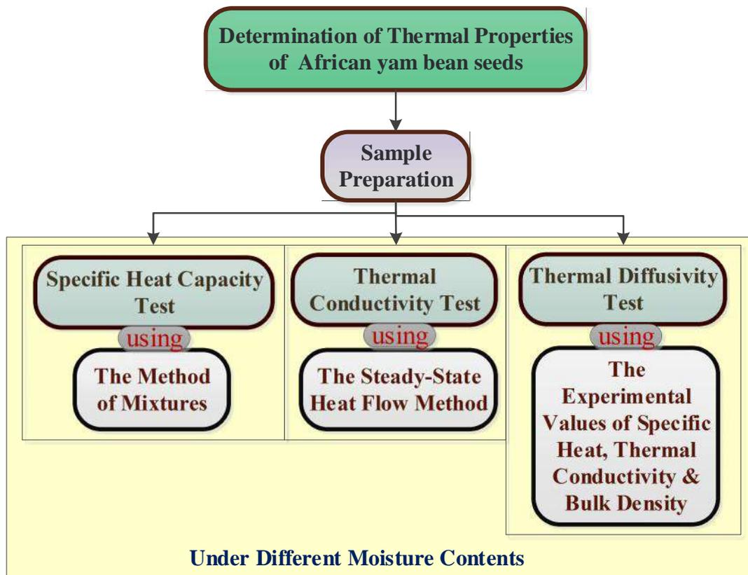
**Figure 1: Test program for determining thermal properties of African yam bean seeds under different moisture contents**
