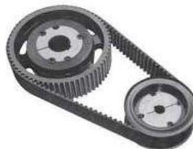
The whole mechanism drives by the DC motor through the timer – pulley – belt power transmission mechanism. Here , the main purpose of timer belt is to reduce/prevent the slippage phenomenon , whereas pulleys with different diameter used to reduce RPM from 100 to 34 . Smaller pulley engaged with the motor output shaft & bigger one is engaged with the extruder & drives the extruder to forced out the product through the well shaped dice.
