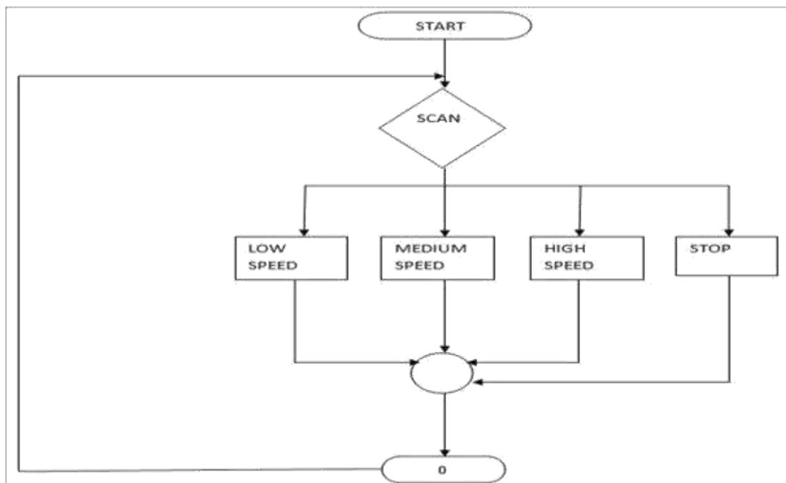
FIG . 1 SPEED CONTROL FLOWCHART
