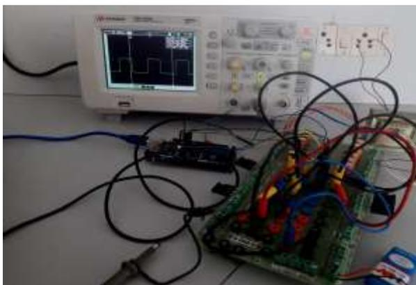
Fig. 9. Working model of symmetric five level cascaded inverter
