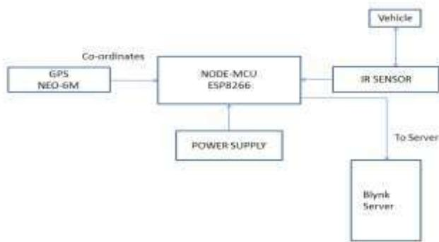
**FIG 2: BLOCK DIAGRAM OF SMART PARKING**
