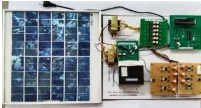
Fig.7. Prototyped model of PV based 13 level inverter
