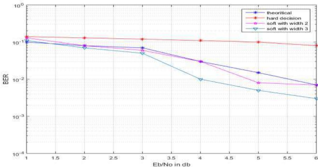
**Figure 8: Comparison soft decision coding with width 2 and soft decision coding with width 3**
