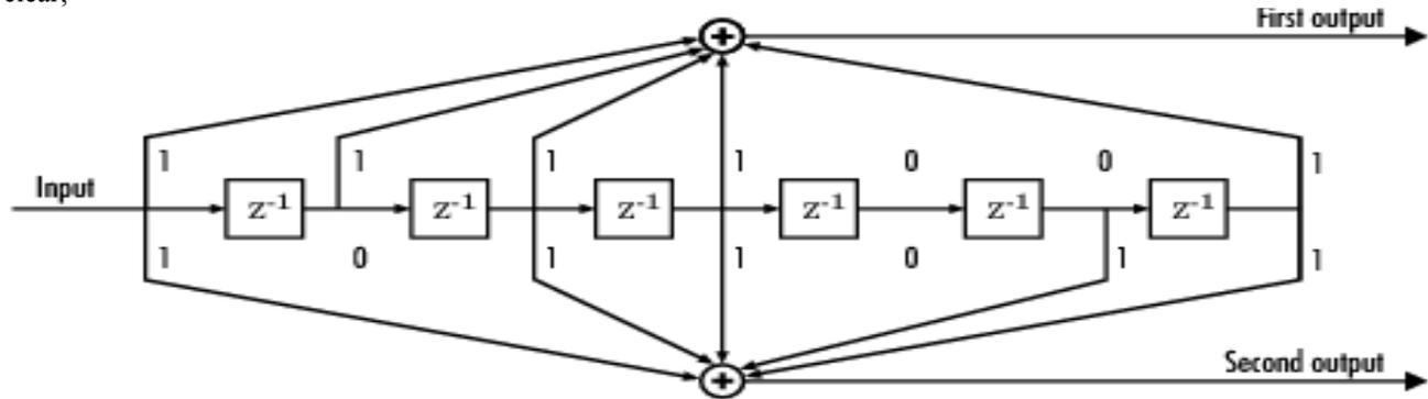
**Figure 2: A convolutional Encoder of Rate 1/2, Constraint length 7.**
