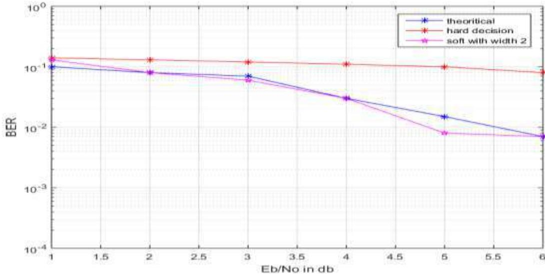
**Figure 6: BER vs SNR curve of different quantization widths for rate 1/2 Binary Convolutional Encoder**
