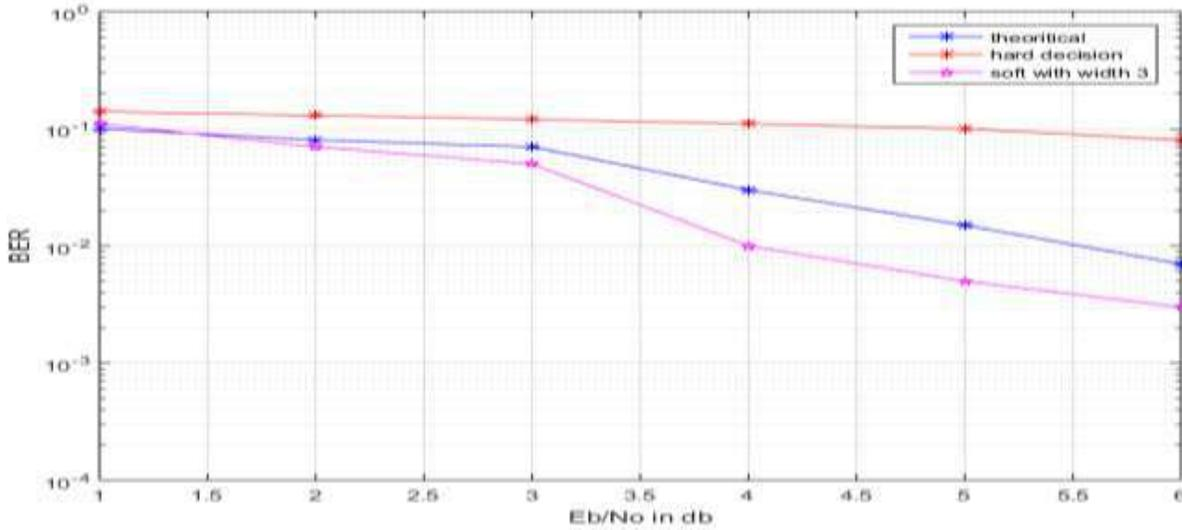
**Figure 7: BER performance of rate 2/3 convolutional encoder showing curves for different quantization widths with soft decision decoding.**
