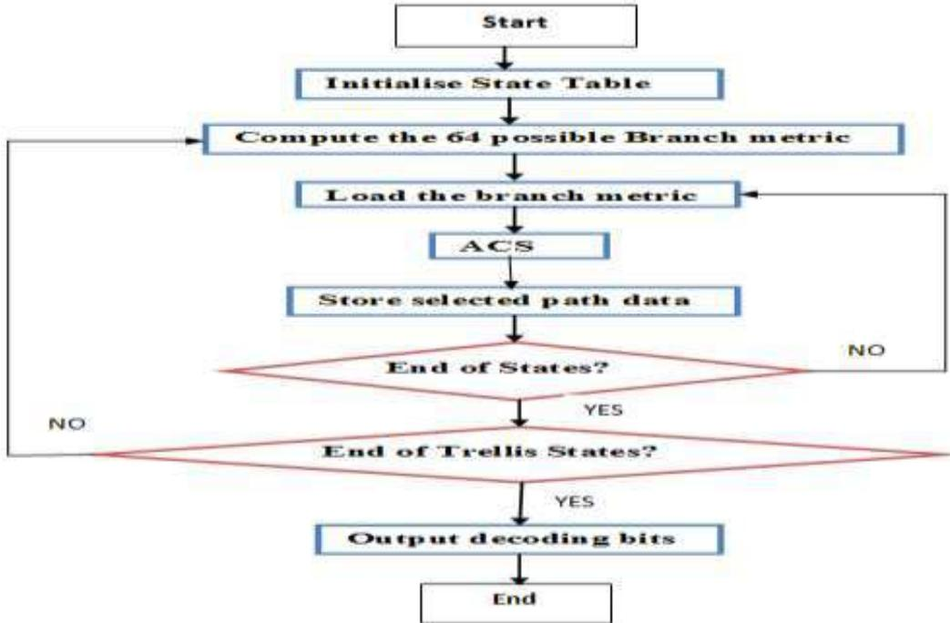
Figure 4: Flow diagram of Viterbi decoder implementation
