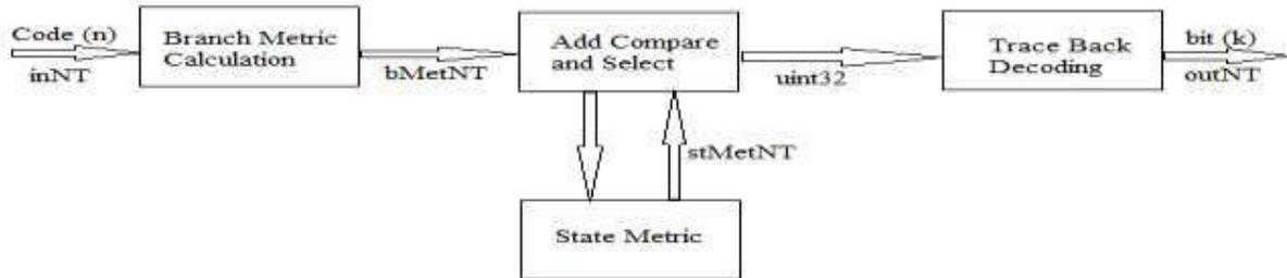
**Figure 3: Viterbi Decoding Algorithm**
