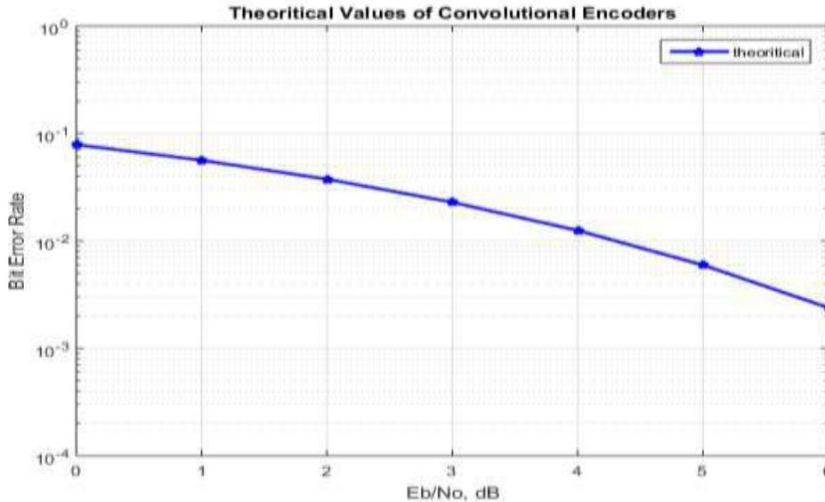
**Figure 5: Theoretical graph of the Convolutional Encoder**
