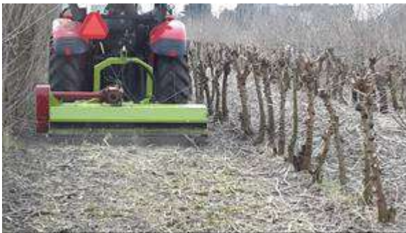
Figure 6. A flail mower chipping cut mulberry shoots.
