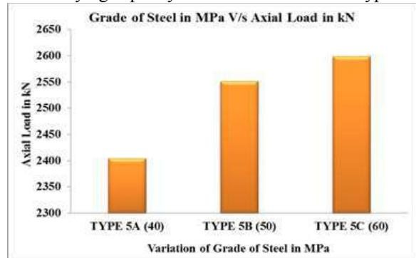
Fig 3.6 Variation of Grade of Steel in MPa v/s Axial Load in kN
