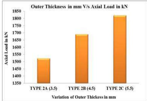
Fig 3.2 Variation of Outer thickness in mm v/s Axial Load in kN
