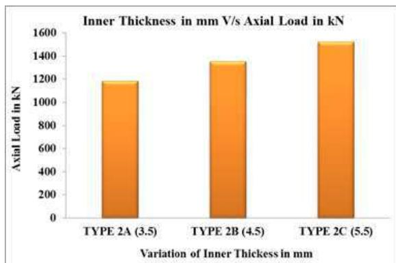
Fig 3.4 Variation of Inner Thickness in mm v/s Axial Load in kN
