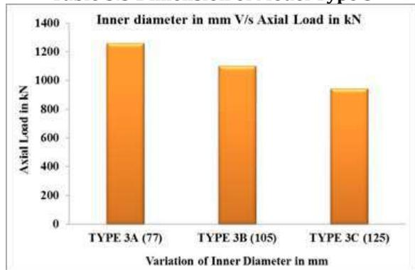
Fig 3.3 Variation of Inner diameter in mm v/s Axial Load in kN
