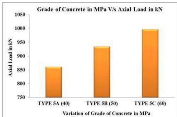
Fig 3.5 Variation of Grade of Concrete in MPa v/s Axial Load in kN
