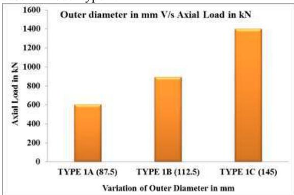
Fig 3.1 Variation of Outer Diameter in mm v/s Axial load in kN
