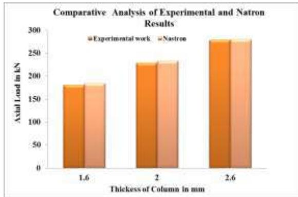
**Fig 3.7 Comparative analysis of Experimental and Nastron results by varying thickness of the column in mm**
