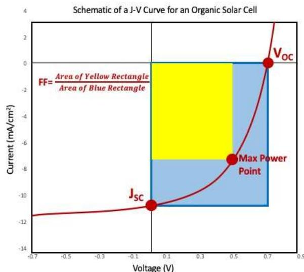
The short circuit current is the maximum photocurrent generation value. It corresponds to the y-intercept value of standard current-voltage curve in which current is
