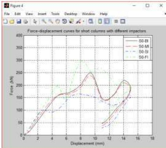
**Fig6: Force-displacement curves for different indenters**
