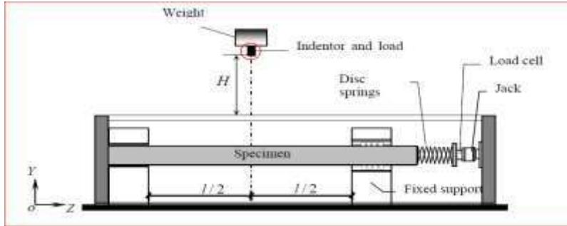
Fig2: Schematic view of test set up
