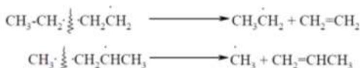
The resulting small radicals react again with the starting molecules. A chain process is developing. Chain termination occurs through the recombination and disproportionation of radicals. The main part of the chain reaction products is formed at the stage of chain development, therefore, the total cracking process of n-
