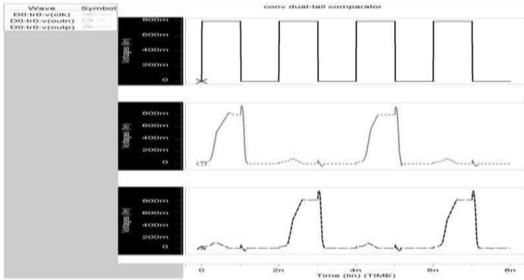
Fig. 9: Simulated Waveform of Comparator 1 (180nm)
