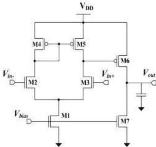
**Fig. 2: Open-Loop Comparator**
