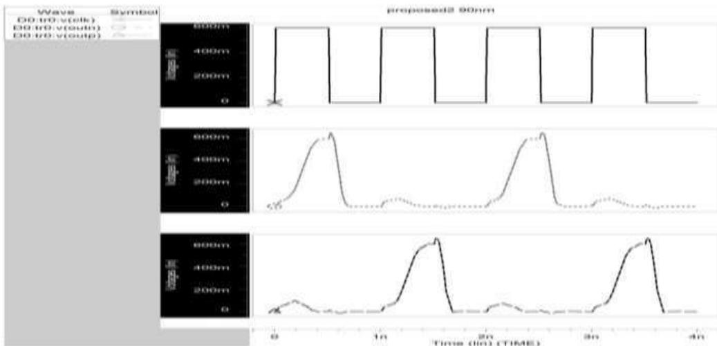
Fig. 14: Simulated Waveform of Comparator 3 (90nm)
