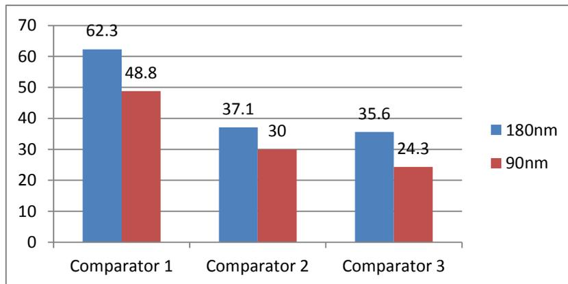
**Fig. 15: Power consumption comparison of dynamic comparators**
