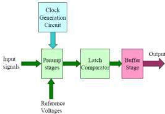
**Fig. 1: High Speed Comparator Architecture**
