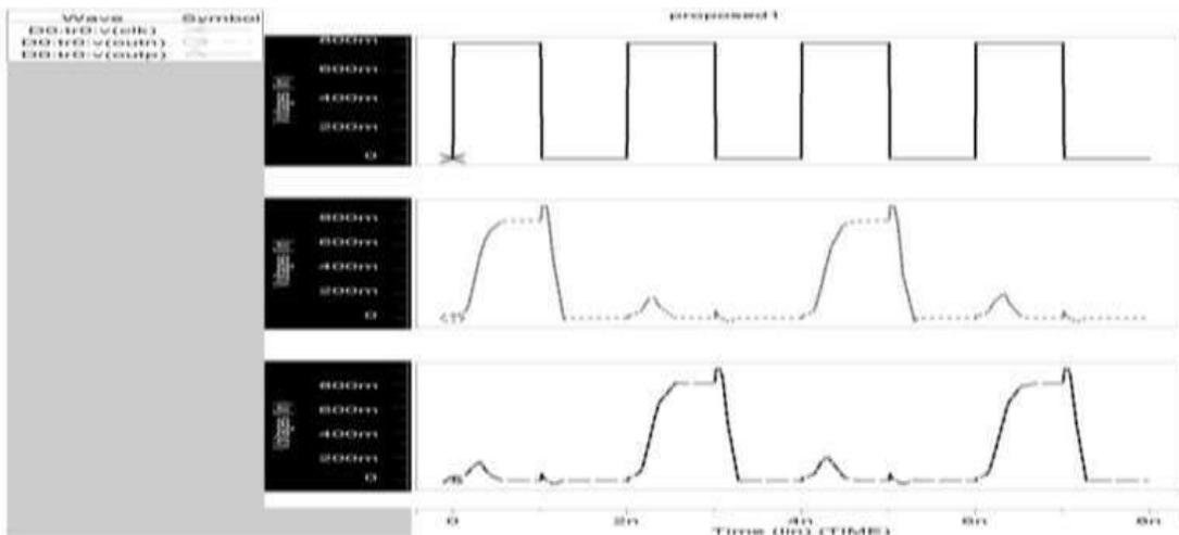
Fig. 10: Simulated Waveform of Comparator 2 (180nm)
