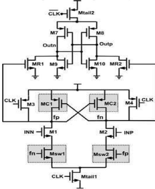
**Fig. 5(b): Final Structure of the Proposed Comparator (Comparator 3)**
