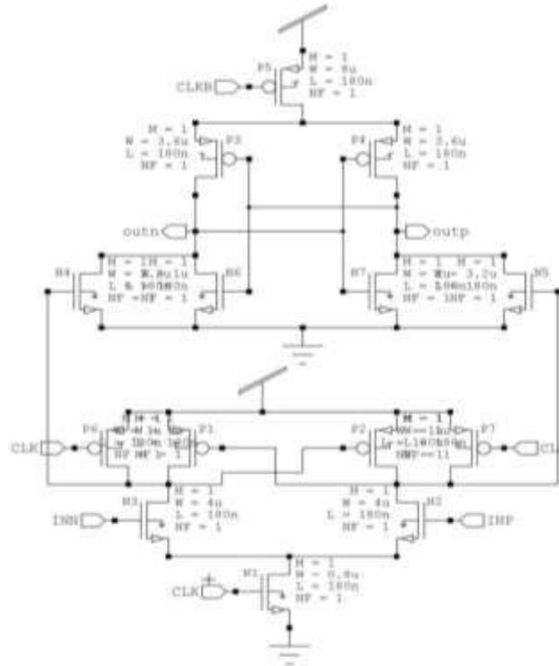
Fig. 7: Schematic of Proposed Comparator (Comparator 2)
