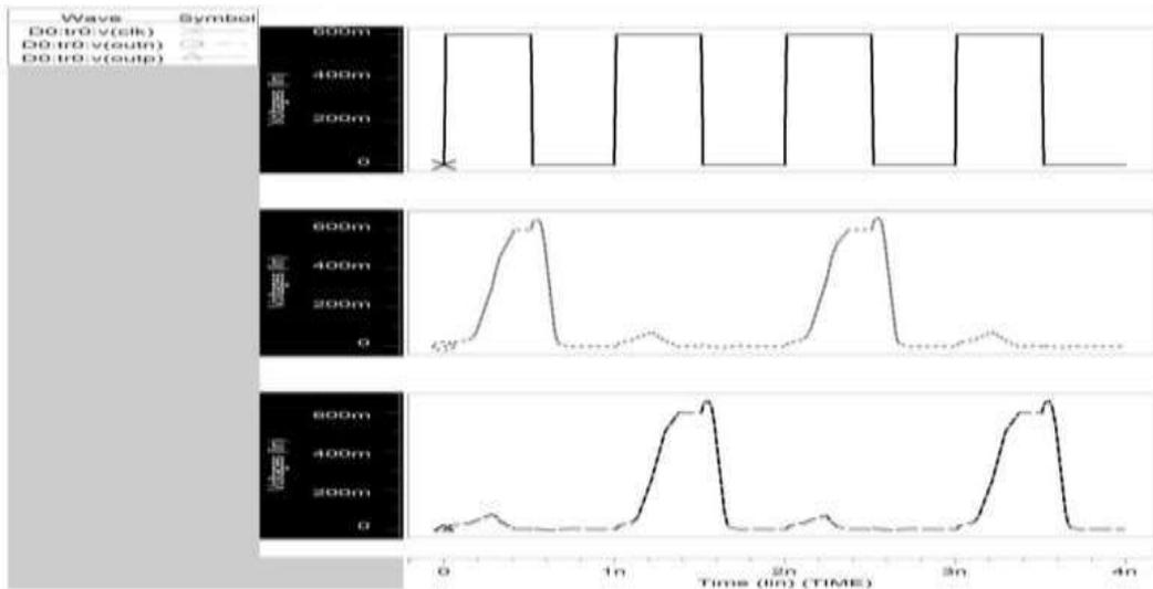
Fig. 13: Simulated Waveform of Comparator 2 (90nm)
