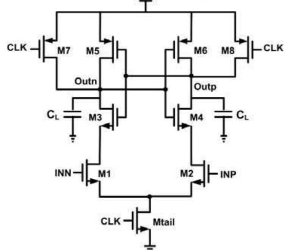
**Fig. 4: Conventional Dynamic Comparator (Comparator 1)**
