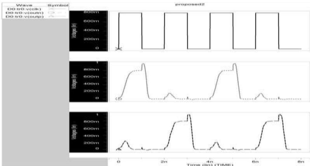
Fig. 11: Simulated Waveform of Comparator 3 (180nm)
