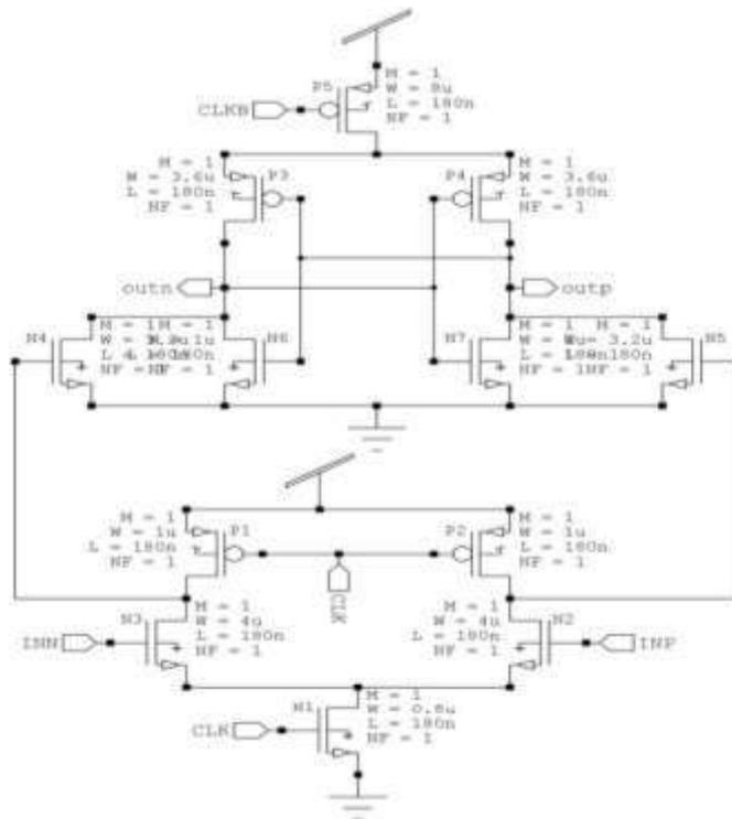
**Fig. 6: Schematic of Conventional Dynamic Comparator (Comparator1)**
