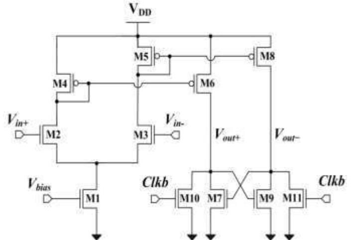
**Fig. 3: Pre-Amplifier Based Latched Comparator**
