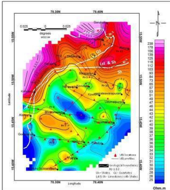
Figure 2. Contour map of apparent resistivity, AB/2=5m, of Panyam study area along with VES locations and profiles.
