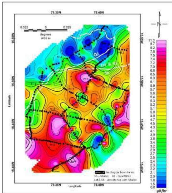
**Figure 3. Radiometric contour map of Panyam mandal, along with radiometric profiles.**
